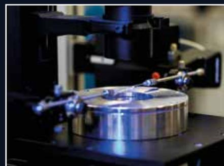
*Flow assurance research: Micromechanical force apparatus allows measurement of forces between hydrate particles*
