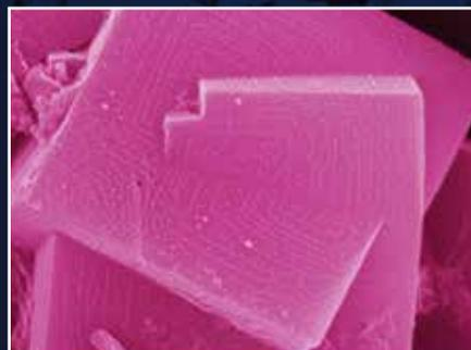
*Gas Separation Research: SEM image of a typical zeolite 3A molecular sieve (standard natural gas dehydration adsorbent) synthesized from coal fly ash in our laboratory.*
