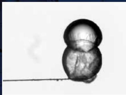
*Flow assurance research: Contacting hydrate particles using the micromechanical force apparatus*
